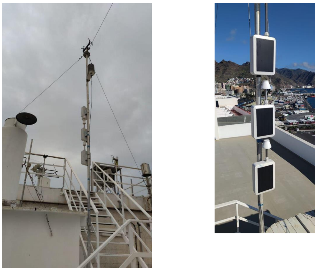
Figure 1: (a) Location of the three DUST sensors at the roof of AEMET's Headquarters measuring collocated with the Micropulse Lidar MPL belonging to MPLNet-NASA network (dome at the left) and the Cimel CE318-TS photometer belonging to AERONET-NASA network (on the right). (b) View of the three DUST prototypes installed in Santa Cruz.
