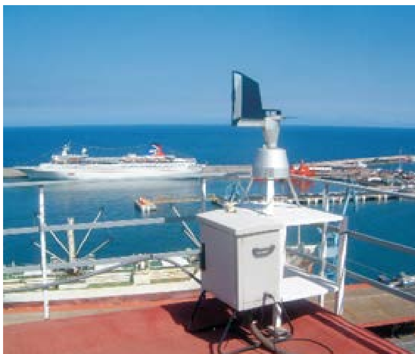
Figure 8.5.1. Hirst, 7-day recorder VPPS 2000 spore trap at SCO, Santa Cruz de Tenerife
