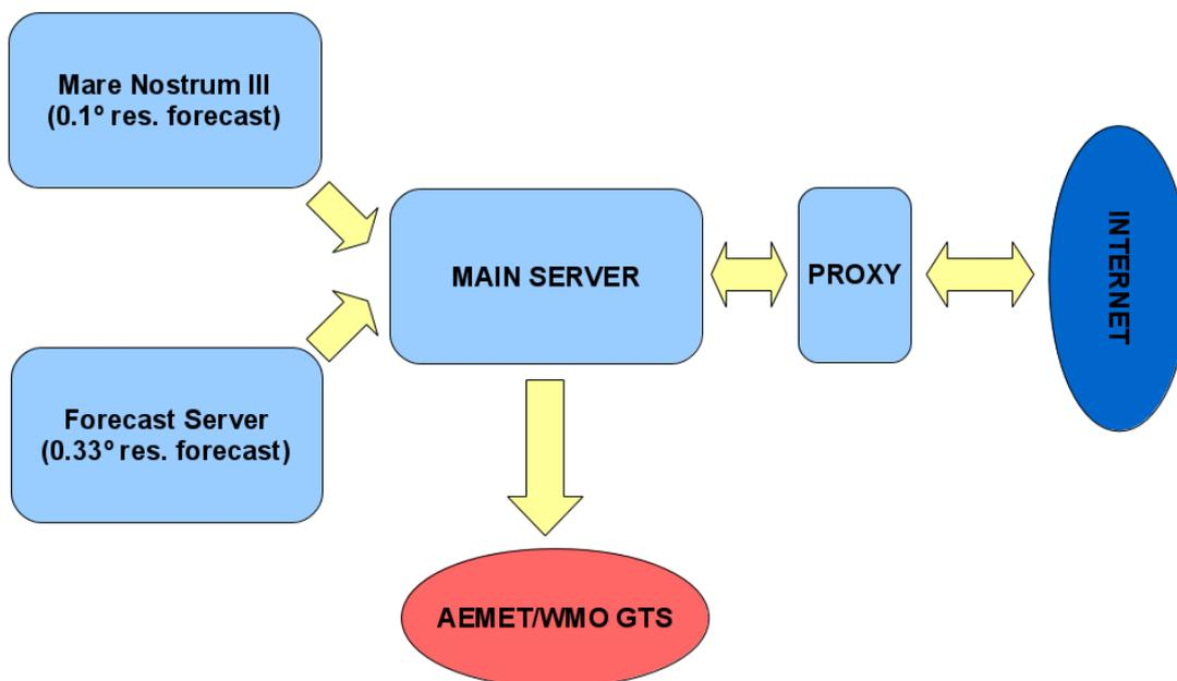
*Figure 2 System architecture of the BDFC.*
