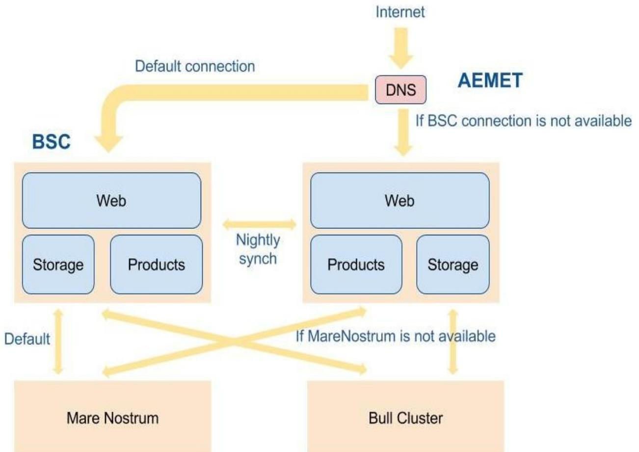
Figure 3: Configuration of the BDFC systems
