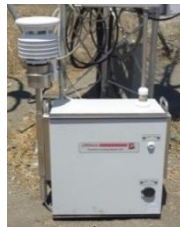
Grimm EDM164 Particle counter
