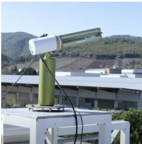
Photometer points at Sun and measures radiance at different wavelengths.
