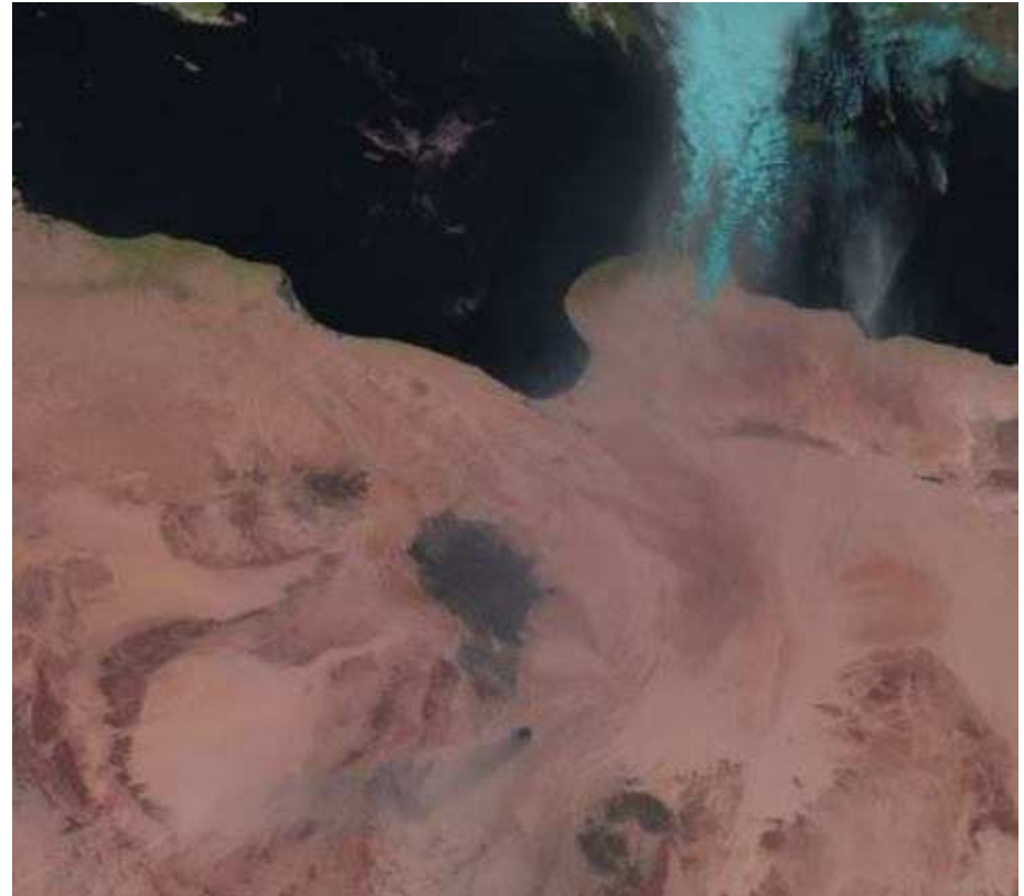
Solar RGB composite based on channels at 1.6, 0.8 and 0.6 \mu\text{m}
